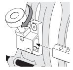
The Extension length is adjustable in increments of 12.7mm (1/2"). Please adjust the Extension length based on the size of your scope housing, and the range of distances you intend to shoot.
