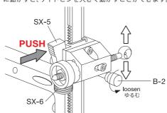
\*\*Please depress the release lever fully when making. adjustments. Not doing this might result in excessive wear to the Worm Gear.
