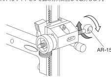
3 Turn Aperture Block sideways as shown, and screw in new sight pin.
