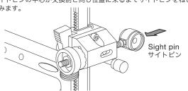
7 Replace SX-8-1 spacer and SX-10 cap screw.Tighten cap screw using the supplied 2.5mm hex wrench.
