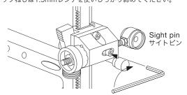
After replacing sight pin, make some shots at close distance, and verify the position of your sight pin is the same as before.
