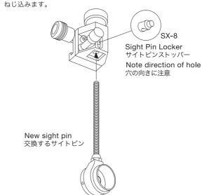
▲ Screw new sight pin through SX-8 Sight Pin Locker. Make sure Sight Pin Locker is oriented correctly.
