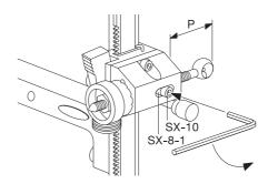
2 Twist AR-15 sight pin in the direction indicated direction to remove.
