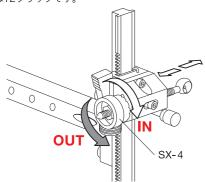
Stop making adjustments in the "OUT" direction when the SX-10 cap screw touches the Polycarbonate Aperture Block as shown. Attempting further adjustments may result in
